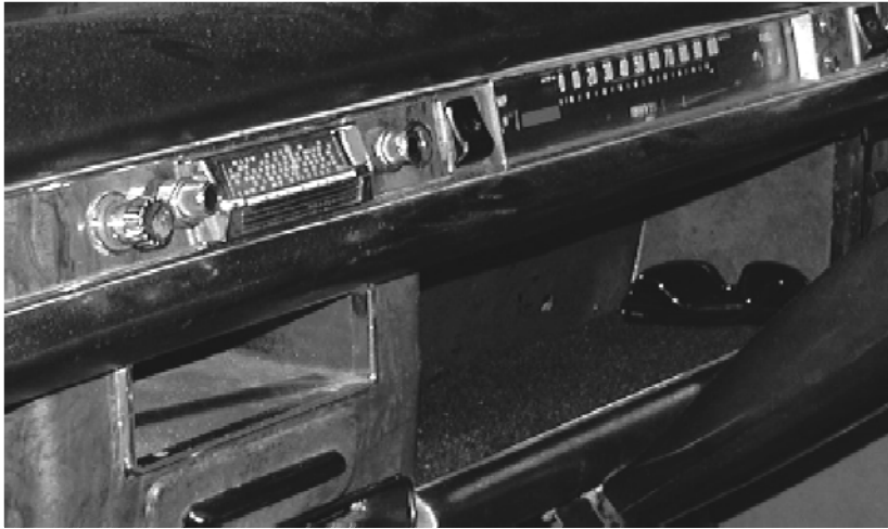
Fig. 3. 8 transistor model fitted to the author's Austin 1800.
